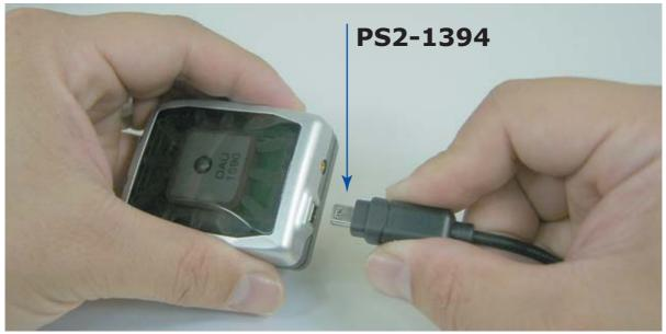
By connecting to different optional connecting cables, HI-406BT-C can be a wired PS/II GPS receivr and used with all kinds of mobile devices.
